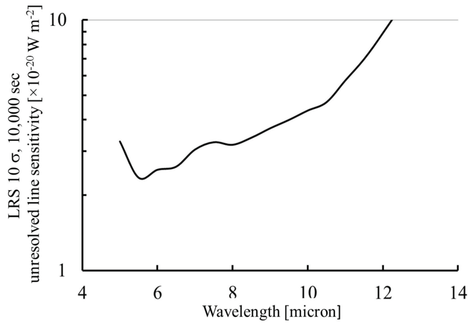
Fig. 12.— LRS limiting sensitivity for the detection of a spectrally and spatially unresolved target (units of 10^{-20} Watt m^{-2} ).
