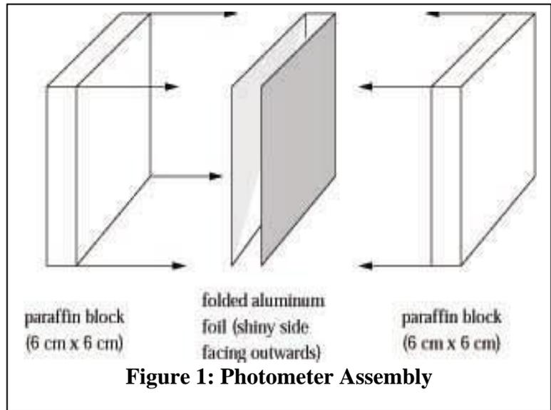
**Figure 1: Photometer Assembly**
