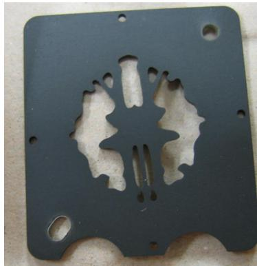
**Figure 4.** Optimized coronagraphic diaphragm. Its transmission is 53 %.
