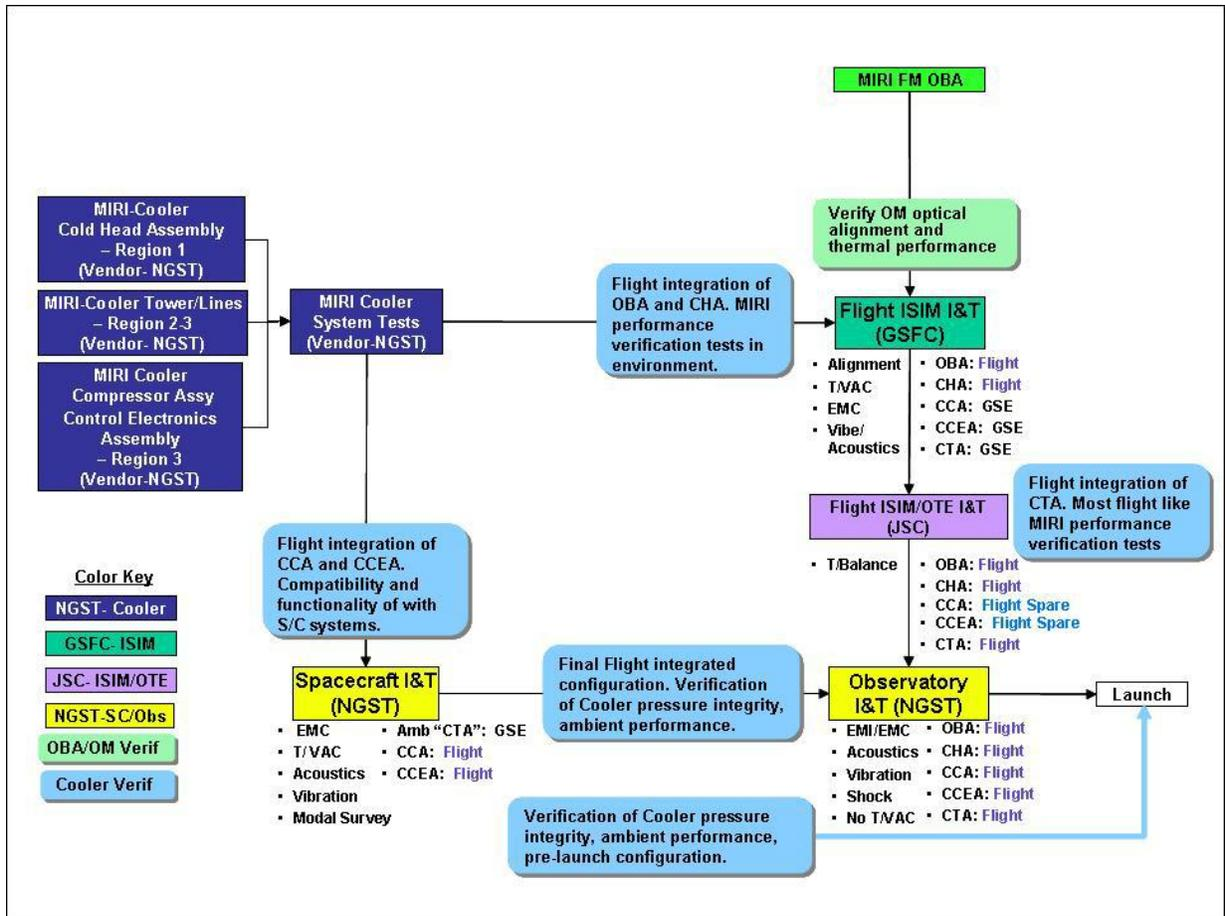
Fig. 5. MIRI Cooler I&T Flow
